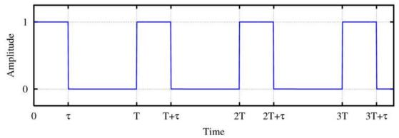
Figure 1: A rectangular waveform
